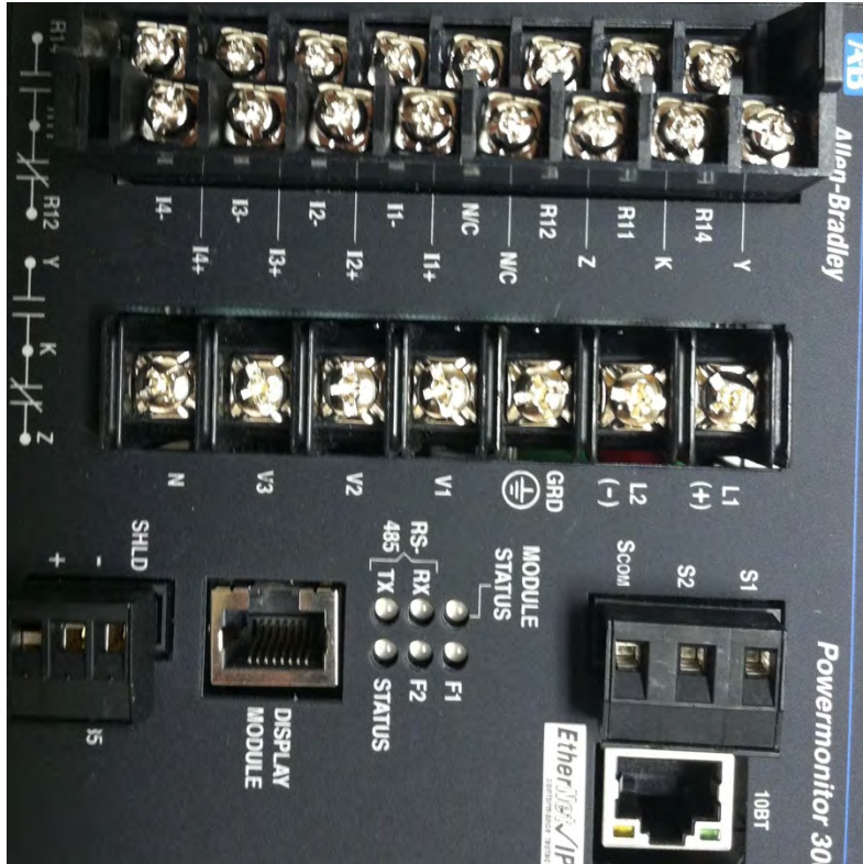
Figure 3.24: Rear termination points on an Allen-Bradley Power Monitor
